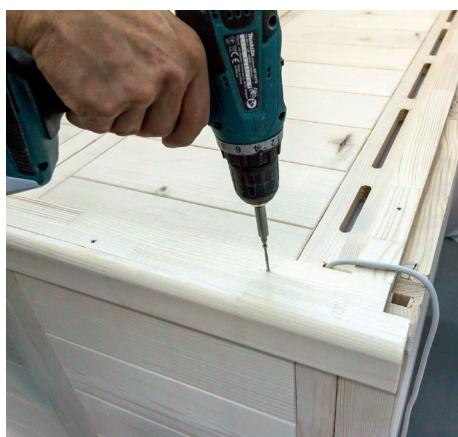
3 mm drill bit, 14 screws 3 x 40 mm
