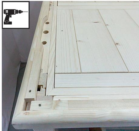
3 mm drill bit, 10 screws 3 x 40 mm
